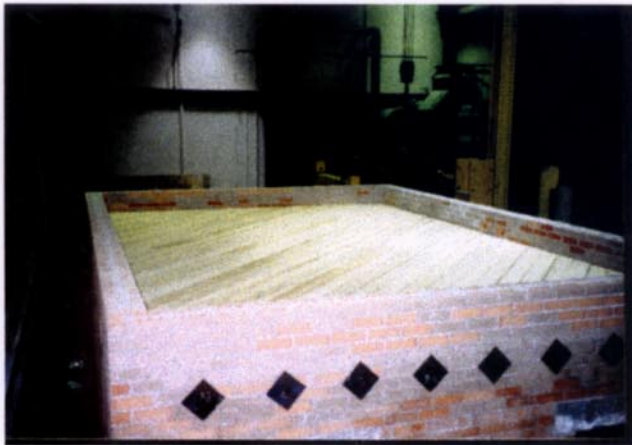
Figure 2: Anchored wood floor diaphragm
